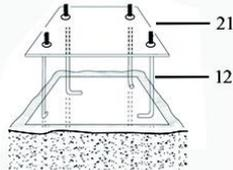
STEP B:fix bottom pole (1) on the inground plate(21)as shown
