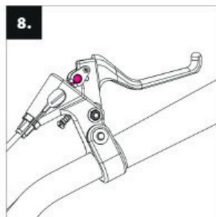
**8.** **Installation of brake cables:** press the brake lever to the maximum and insert the ending of the brake cable into the circular fixing point. Repeat the action with both brakes.
