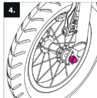
**4.** Tighten both nuts and return the brake cable into the holder.
